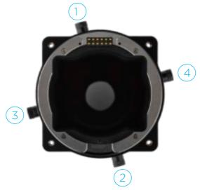
8. Tighten the locking screws with a 2 mm hex tool using a torque of 20 cNm.
