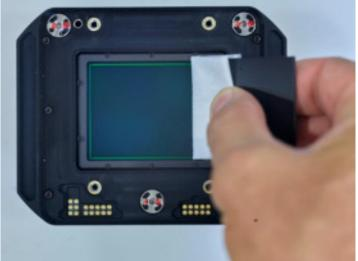
If necessary, move the cloth layer one centimeter on the wiper and repeat the process. Never swipe twice with the same area of the cloth.
