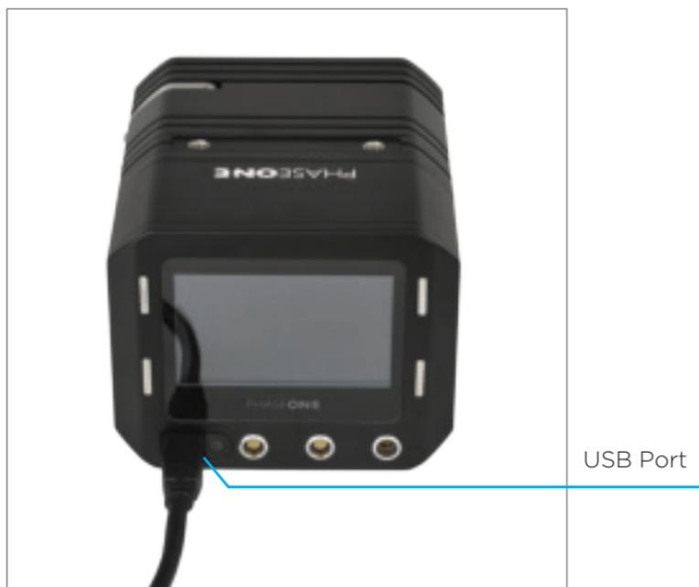
1. Insert the end of the USB 3.0 cable to the USB 3.0 port of the camera.
