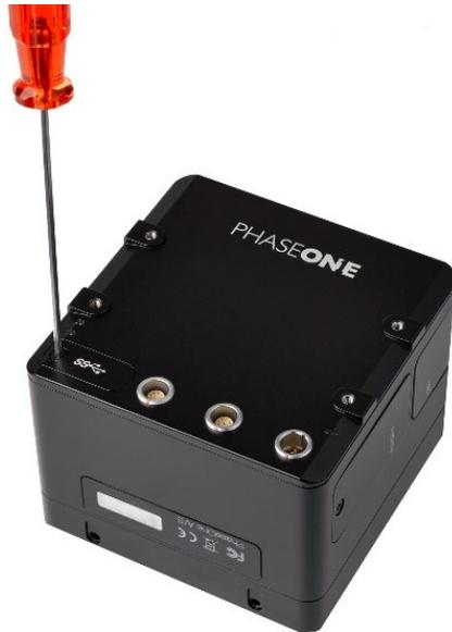
**Figure 16:** Unscrewing USB port cover
