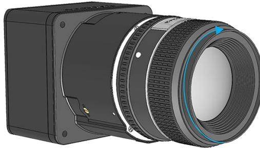
6. Use a flat screwdriver to lock each of the three lens adapter clamp cams by rotating each cam clockwise 90 degrees
