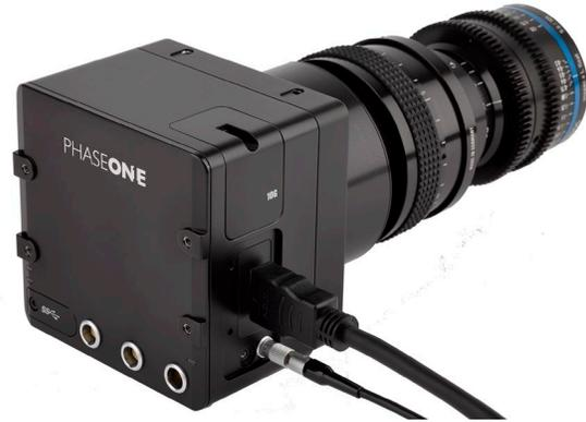
Figure 19: Strobe Trigger Cable & HDMI cable
