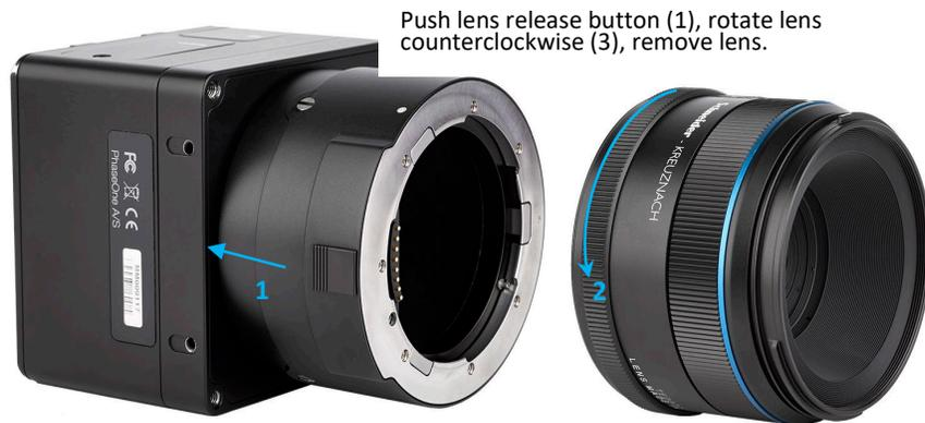
**Figure 13:** Dismounting Lens from SK Lens Adapter
