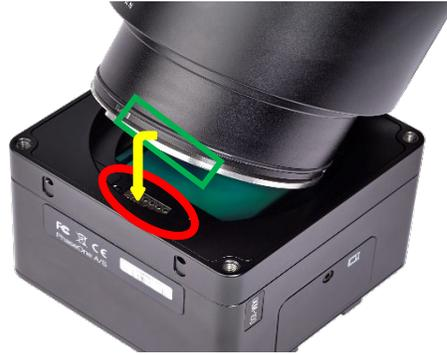
5. Hold the lens with both hands and press it firmly down onto the iXM camera interface, so that the O-Ring seal is pressed inside.
