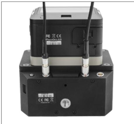
3. Insert a LEMO-secured Phase One control cable into data terminal B (right data terminal).
