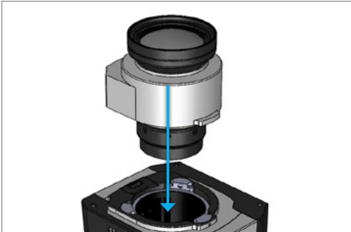
2. With a 2 mm hex key, secure the lens assembly onto the iXA-R by gently tightening each locking screw.
