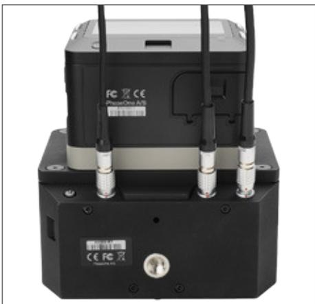
4. Connect the other end of the Phase One control cable into your Flight Management System.
