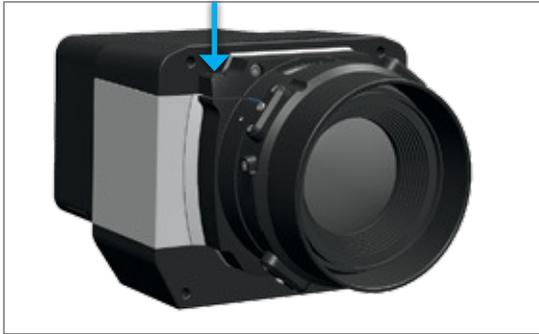
11. Unscrew and remove the Secure Lens Holder covers (shown in blue) on either side of the lens focusing ring with a hex tool.
