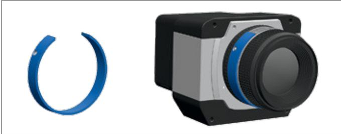
8. Check to make sure that the clamping and Locking screws are not tightened. Slide the back of the Secure Lens Holder over the front of the lens, aligning the lens distance scale in the distance scale window of the Secure Lens Holder. Push the Secure Lens Holder as far as it can go onto the lens so there is no gap between the Secure Lens Holder and the camera.
