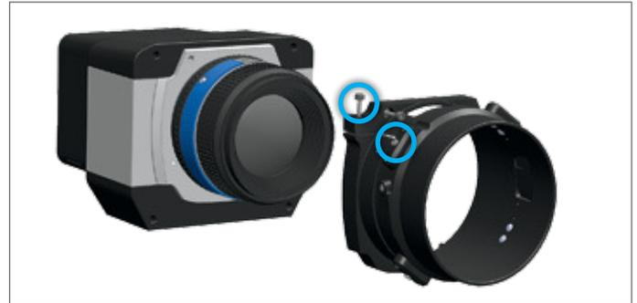
9. Tighten both Lens holder screws into the threaded holes on the front of iXA camera with a hex tool using a torque of 75 cNm.
