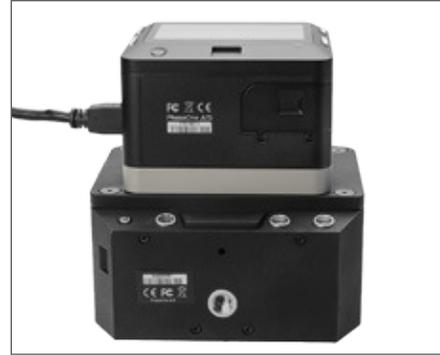
2. Connect the other end of the USB 3.0 cable into a USB port on an iX Controller or the back of your onboard computer or laptop.
