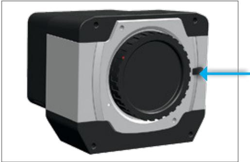
2. Rotate the front body cap counterclockwise and lift out.
