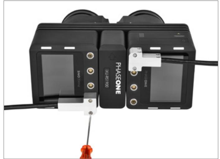
5. Connect the other end of the USB 3.0 cable into the USB port of your iX Controller or on the back of your onboard computer.
