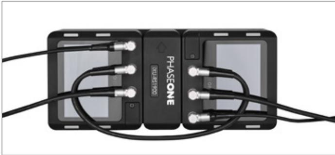
5. Connect an iXU RA multi-sync cable (not included in the box - should be purchased separately) to data terminal B of the second sensor module (right sensor module).
