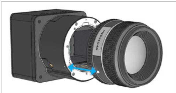
4. Put a body cap on the camera to protect it or place another lens on the camera.
