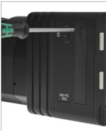
1. With a 2 mm hex key, unscrew the screw on the CF cover.
