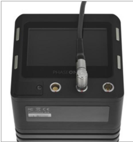
Note: The two data terminals are not interchangeable. Connect devices to data terminal A or B depending on the specific device. See details in "Connecting Control Cables to Devices" on page 34 and "Activating iX Link" on page 46.
