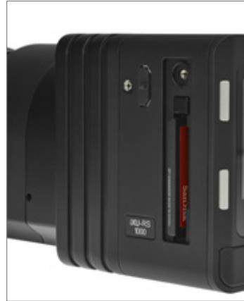
3. Insert a CF card with the brand label facing the display end of the camera as shown in the image.
