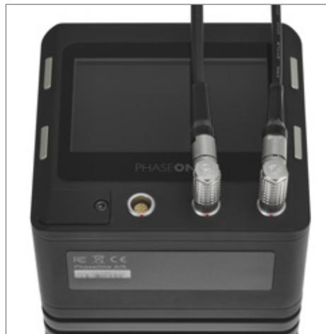
3. Insert an iXU RA control cable into data terminal B (right data terminal).
