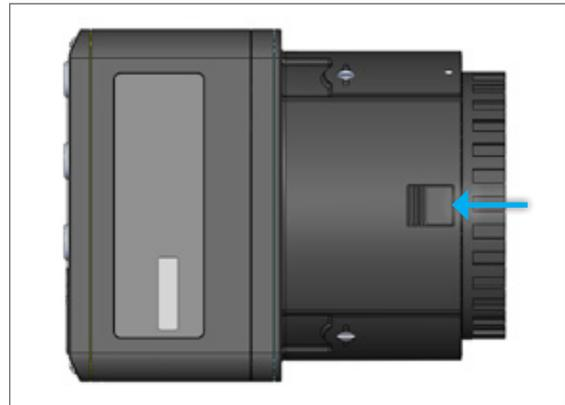
3. Rotate the lens counterclockwise and lift out.
