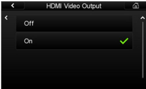
2. From the HDMI Video Output screen select Off. The Menu screen appears with HDMI Video Output Off displayed.
