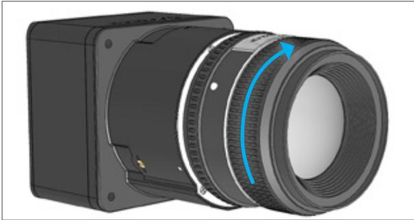
6. With a flat screwdriver, lock each of the three lens clamp cams by rotating each cam clockwise 90 degrees.
