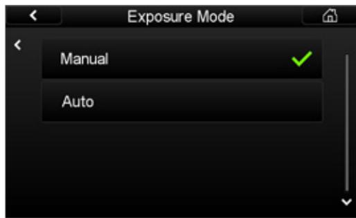
2. From the Exposure Mode screen, tap Auto to activate auto exposure mode or Manual to deactivate Auto Exposure mode.
