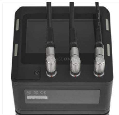
4. Connect the other end of the iXU RA control cable into your Flight Management System and / or a controller using iX Link.
