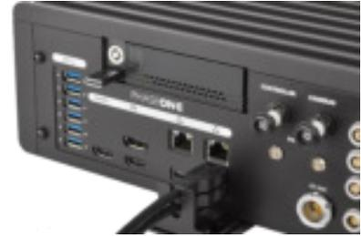
**Note:** The bottom plate of the USB 3.0 cable bracket has two sets of holes for attaching to the iX Controller.
