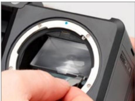
4. When installing a new focusing screen, grasp the tab of the new screen with the tweezers, and place it onto the frame. When performed correctly, the focusing screen should easily settle into the frame. Make sure that the tab is on the right side, otherwise the focusing screen will be upside down.
