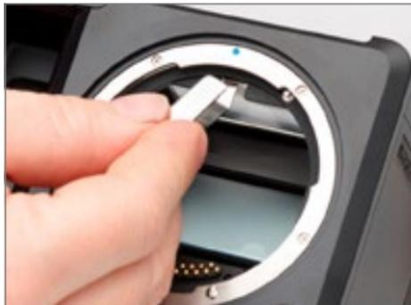
6. Press the frame upwards into position near the release lever until you hear a clicking sound. The screen is now properly installed.
