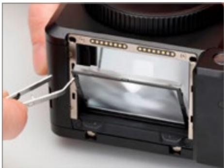
6. Push the screen frame upwards by pressing the tweezers against the corner of the frame.
