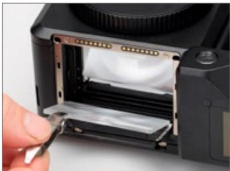
5. When installing a new focusing screen, grasp the tab of the screen with the tweezers, and place the screen onto the frame and as far as possible into the back end of the frame. Make sure that the tab is on the left side, otherwise the focusing screen will be upside down.
