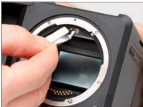
1. Remove the prism viewfinder or waist level viewfinder from the XF camera body. This will make it much easier to see inside the mirror box.
