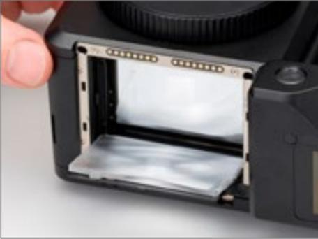
3. Continue with the tilting movement until the focusing screen follows the frame down, then rest the camera body on its back.
