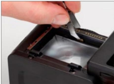
1. Remove the digital back and lens from the XF camera body. Next, remove the prism viewfinder or waist level viewfinder from the XF camera.
