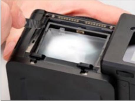
7. Slowly tilt the XF camera body to its upright position, while keeping the tweezers against the frame, as shown.
