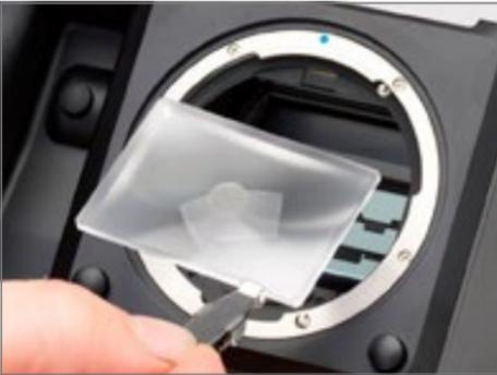
3. Carefully remove the focusing screen from its frame by grasping the tab on the edge of the screen with the tweezers. Make sure that you do not scratch or touch the focusing screen or the mirror while removing it from the mirror box.
