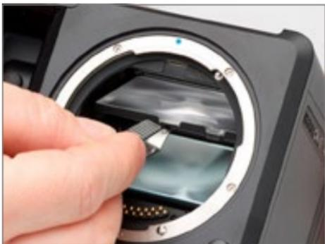
5. Push the screen frame upwards using the tweezers, while being careful not to touch the focusing screen or the mirror.
