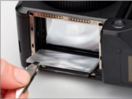
4. Carefully remove the focusing screen from its frame by grasping the tab on the edge of the screen with the tweezers. Make sure that you do not scratch or touch the focusing screen while doing so.
