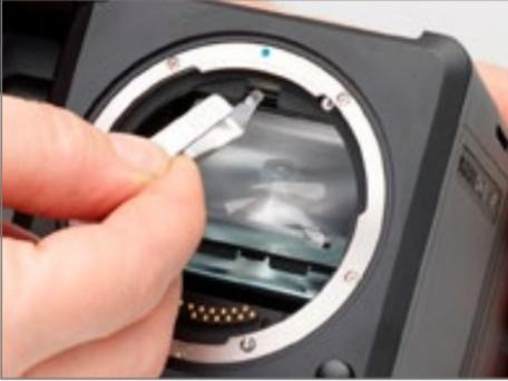
2. This will release the frame, and the focusing screen will drop down in the mirror box.
