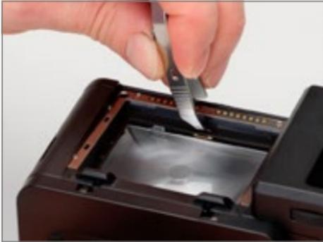
8. Finally, press the frame downwards close to the screen release lever until you hear a click. The screen is now properly installed.
