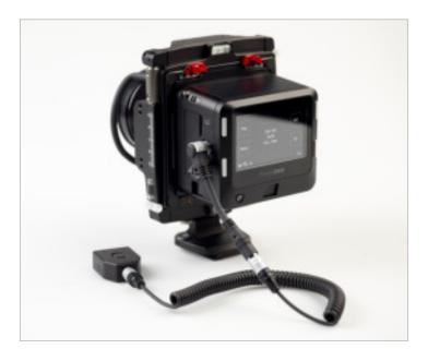
The remote release units made to work with the XF Camera use a 12-pin multi-connector port while the IQ3 Digital Backs only accept an 8-pin connector. The Cable Release Adaptor (part number 73174) ensures compatibility by plugging it into the 8-pin multi-connector port on the side of the IQ3 Digital Back, while the other end of the adaptor accepts both a 12-pin and an 8-pin connector.
