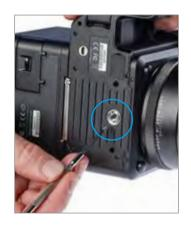
Use the supplied screwdriver and remove the small retaining screw from the tripod mounting socket of the XF camera body. Make sure to store the screw a safe place, as you will need it again if you want to secure the tripod thread adapter later on.
