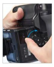
Press the V-Grip against the XF camera and turn the quick release latch 90 degrees up in order to lock the V-Grip securely into place. Please make sure that the safety switch locks correctly with a tactile click.
