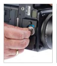
Use the supplied disc or a coin to securely fasten the quick release adapter or L-Bracket, turning it clockwise.
