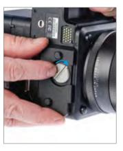
Place the supplied quick release adapter or L-Bracket over the tripod mount so that the screw and pins align with the holes in the XF camera body. Tighten the screw by placing it in the groove and turning the head clockwise.
