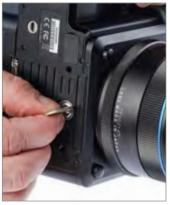
Use the supplied disc to remove the 1/4" - 3/8" thread adapter screw from the XF camera body's tripod socket by turning it counterclockwise.
