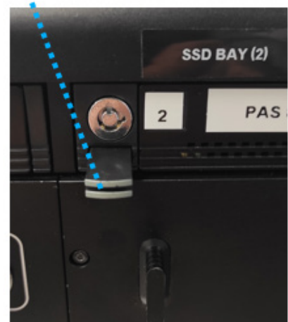
SSD carrier eject button
