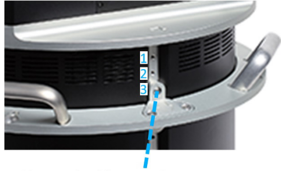
Example: T-mount upper screw is inserted into hole No. 3 from top of vertical rail
