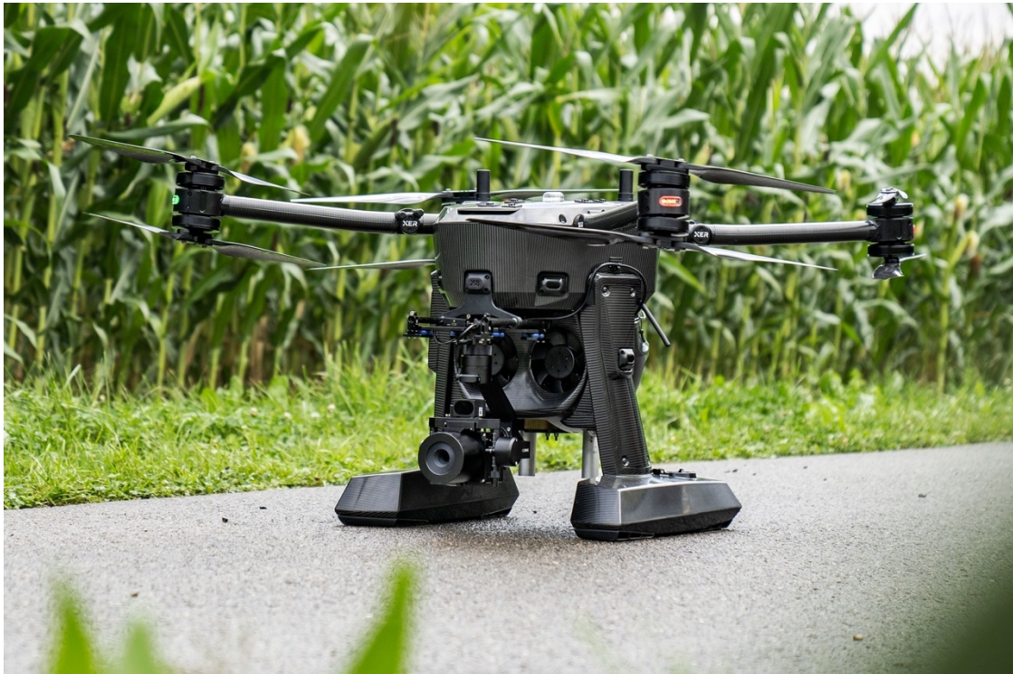
Photo: Close-up of the integration of the Xer X8 UAS and Phase One P3
