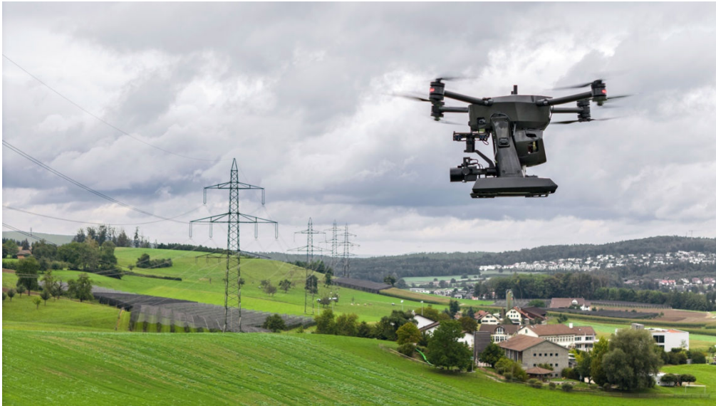
Photo: Automated long-range powerline inspection with the Xer X8 UAS and Phase One P3
