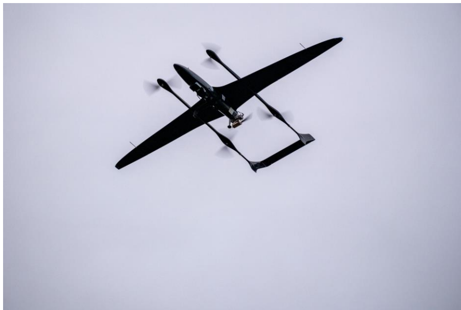
The Carbonix Ottano X flying with RIEGL VUX-120 and PhaseOne IXM-100
