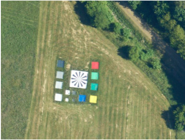
Figure 2 Siemens Star target in the test area
