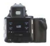
**Above:** When you turn on the IQ2 backs, you are greeted by an opening screen similar to this one for the IQ280. The touch screen displays icons for the four buttons surrounding the screen. You can navigate using the touch screen or the buttons.
